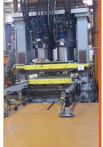
Tests have been performed applying different values of vertical load, in order to simulate a more or less loaded rack, and at different velocities.
