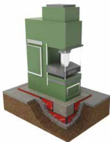
Example of inertial inertial application in the pit. MEGAMAT line
