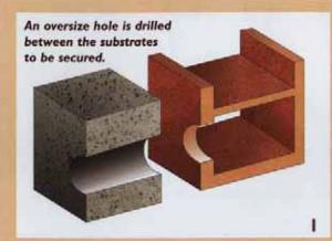
The Cintec system comprises a steel section in a mesh fabric sleeve, into which a specially developed cementitious grout is injected under low pressure. The flexible sleeve of woven polyester restrains the flow and moulds the anchor into the shapes and spaces within the walls, providing a strong mechanical bond.
