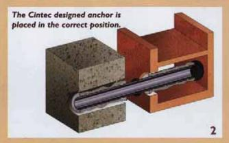
The anchor is inflated like a balloon to provide a permanent cementitious anchoring solution using one of Cintec's range of sympathetic grouts.
