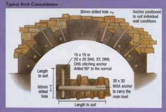
CHS - Circular Hollow Section ST - Stud RAC - Remedial Anchor Cavity DRB - Deformed Rib Bar SHS – Square Hollow Section WSA – Wall Supporting Anchor
